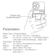
REMARK: When using any two Port outputs (including wireless charging) at the same time, the fast charging mode (9V/ 12V) will be closed automatically and product will enter the normal charging mode (5V), the wireless switch to 5W automatically.
